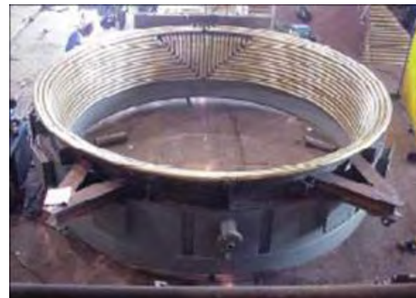
Al-Bronze Skirt Prior to Installation
